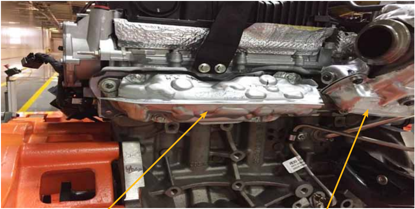
Exhaust Assembly Heat Shield assembled on vehicle engine.
